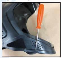
1) Using a thin tool, such as a flat blade screwdriver, insert near edge to pry the current chin guard free from the helmet.
